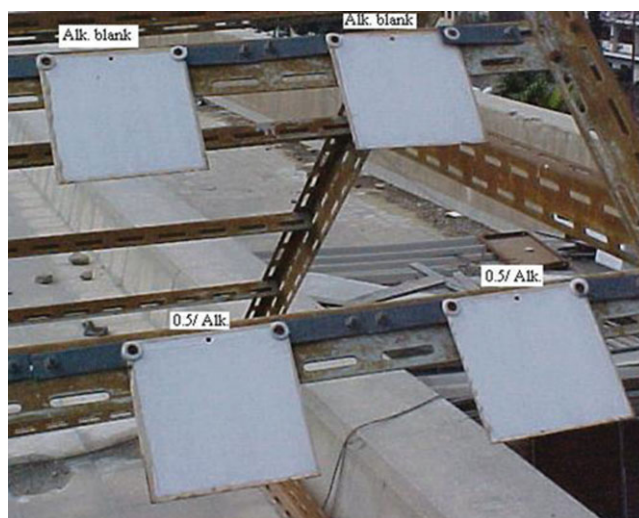
Figure 8 Alkyd coated test panels after 6 month exposure. [Color figure can be viewed in the online issue, which is available at www.interscience.wiley.com .]
